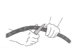
Flexible polyethylene plastic pipe is very easy to work with. You can cut it with a saw or, shown here, with a sharp knife.
