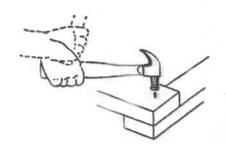
The hammer stroke in driving a nail.
