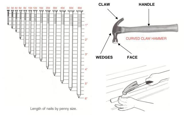
Proper procedure for grasping hammer: Grasp hammer firmly near the end.
