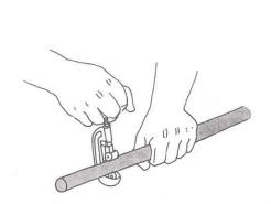
Special pipe cutter for plastic gives good, even cut. Blade on this cutter is narrow to prevent large burrs.
