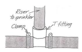
Special adapter T joins polyethylene pipe with threaded galvanized steel pipe (called a "riser") for sprinklers.
