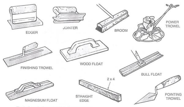
Tools for placing and finishing concrete.
