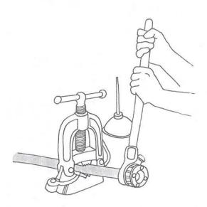
Step 4. Fit pipe threader over pipe end and tighten it. Exert force at first while turning to start cutting action.
