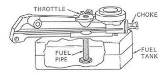
3. Fuel pump (Pulsa-jet). This carburetor uses a diaphragm type fuel pump to keep a constant level in the fuel chamber. (See Figure XI.)
