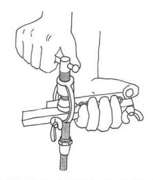
Special flaring tool does precise job. Clamp it down over pipe end and screw tapered head into pipe, creating flare.
