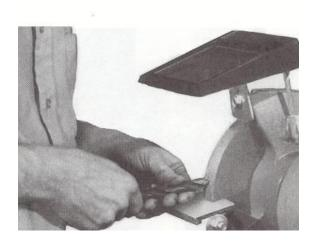
4) While giving a clockwise twist, grind one side to 59°. Rotate bit and grind other side exactly the same. To prevent overheating, frequently dip bit in cool water. After grinding, use toolsharpening gauge to check the angle of lips, position of dead center, and clearance of resharpened drill bit. (See Figure VII and VIII.)
