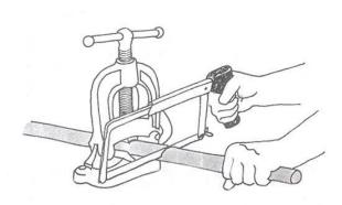
Step 1. Fit pipe into the vise. (Some have pipe jaws under regular jaws.) Cut with hacksaw or a pipe cutter.
