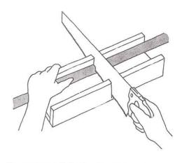
You can also cut plastic pipe with a regular handsaw. To insure a square cut, place it in a miter box, hold securely.
