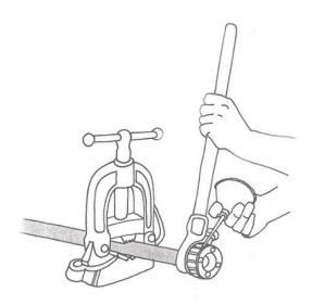
Step 5. While cutting threads, use generous amounts of oil. Chips may stop threader. Back off, brush chips away.
