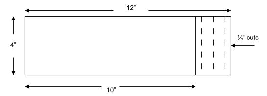
b. Rip the 2" x 4" x 10" board down the center and check for square cut.
