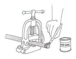
Step 6. Threads cut, pipe end cleaned off, apply pipe joint compound to threads to help seal the completed joint.
