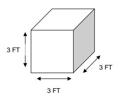
1. Determine the cubic yards of concrete needed by multiplying the thickness by the width and length:
