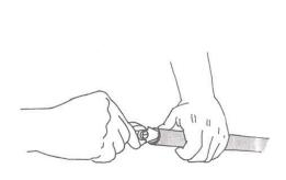
After cutting plastic pipe you'll find burrs, just as on metal. You can remove them with a sharp knife instead of a reamer.
