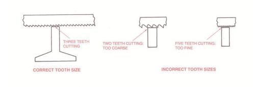
When cutting mild steel or cast iron over 1/8" thick, use a coarse blade (18 teeth per inch). Hard steel, pipe, and heavy sheet metal can be cut with a medium blade (24 teeth per inch). Thin sheet metal tubing should be cut with a fine blade (32 teeth per inch).
