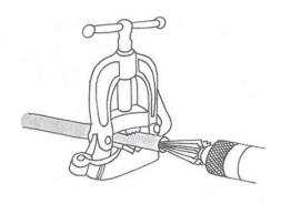
Step 3. File off burrs on the inside of the pipe with a reamer. Vise holds pipe steady during the reaming process.
