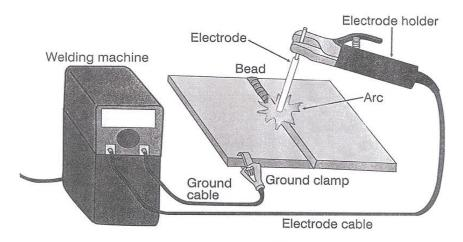
Components of an arc welding system.
