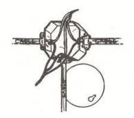
A junction box contains only the splices of several lengths of cable.
