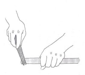
Step 2. Cutting will leave burrs on both the inside and outside of the pipe. File off the outside burrs.
