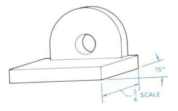
Oblique drawing is a form of pictorial drawing in which the plane of projection is parallel to the front surface of the object. The lines of sight are at an angle to the plane of projection and are parallel to each other. This allows the viewer to see three faces of the object. The front face and any surface parallel to it, is shown in true shape and size, while the other two faces are distorted in relation to the angle and scale used.
