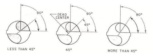
Examples of correct and incorrect angles for sharpening twist drill. (See Figure IX.)
