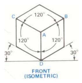
The word isometric means equal (iso) measure (metric). Isometric drawing is a form of pictorial drawing in which the receding axes are drawn at 30° from the horizontal as shown.
