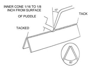
MAKING A CORNER WELD WITHOUT A FILLER ROD.
