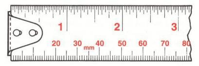
This tape has both U.S. Customary and metric units of measurement. The 1, 2, 3 values refer to inches. The 20, 30, 40 values refer to millimeters.
