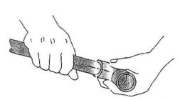
Place titting over the end of the pips (It should fit snugly) and mark both pips and fitting to show exact placement.
