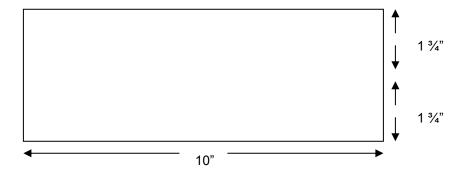
c. Using a block plane cut the 1 3/4" pieces of wood to 1 1/2" x 1 1/2" x 10".
