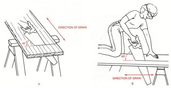
When using a crosscut saw, hold the saw at a 45 degree angle. When using a rip saw, hold the saw at a 60 degree angle. Start all cuts with short strokes, then use full, even strokes for good cuts. The saw kerf should be on the waste side of the line.
