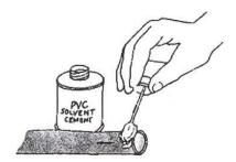
Apply a thick cost of special plastic solvent coment to the outside of the pipe end. It dries fast so don't dawdle.
